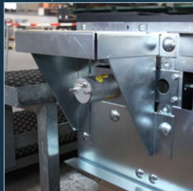
Tachometer for belt speed
